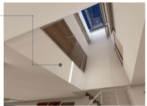
Central lightwell enhancing natural ventilation and daylighting in the kitchen and bathrooms
