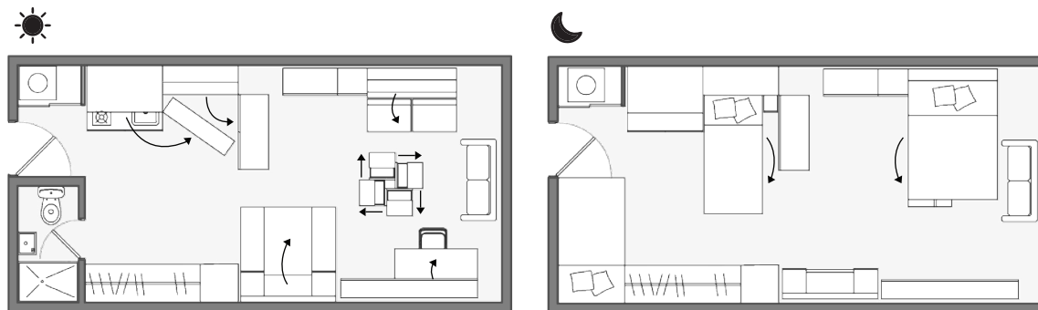
Flexible modules 05 and 06 4 mt x 4 mt each 32 m 2 total Typology: Family, 4 people
